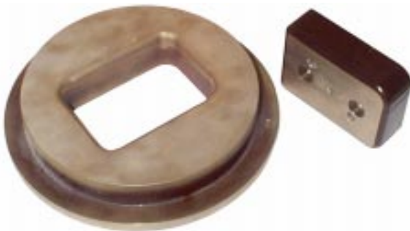
Figure 1: Laser beam sintered tool set (punch and die) for the deep drawing of prototype parts
